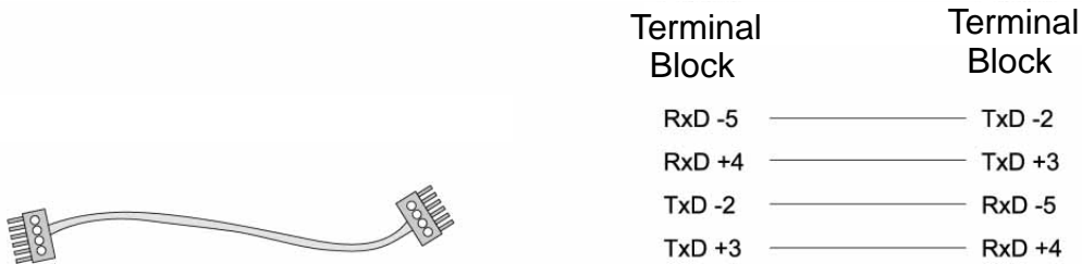
Figure 51: Cable 4 for the TS110/100 - Terminal Block to Terminal Block, crossover full duplex
