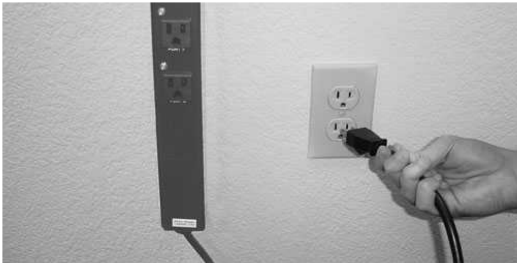
Figure 1: Connecting the AlterPath PM to a power source
