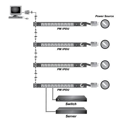
PM IPDU to the chain, connect its In port to the last Out port in the chain. Repeat these steps until you have connected the desired number of PM IPDUs.
