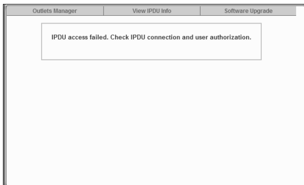
Figure 3.17: IPDU Access Failed Message from Outlets Manager
