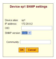
Figure 6-36: Config → SNMP: Device SNMP Access Dialog With V2c Selected
