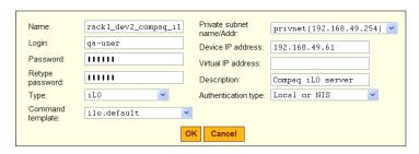
Figure A-4: Example 1: Device Configuration Example
