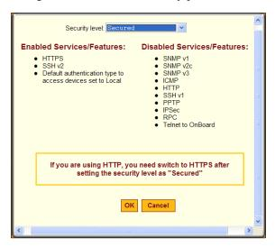
**Figure 6-46:**Config → Security Profile Dialog With the "Secured" Profile Enabled
