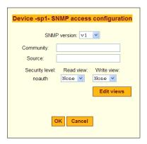
Figure 6-38: Config → SNMP: Device SNMP Access Dialog With V1
