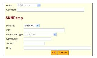
**Figure 6-28:** Config  $\rightarrow$  Sensor Alarms SNMP Trap Fields
