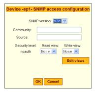
**Figure 6-40:** Config → Device SNMP Settings Dialog With V3 Selected
