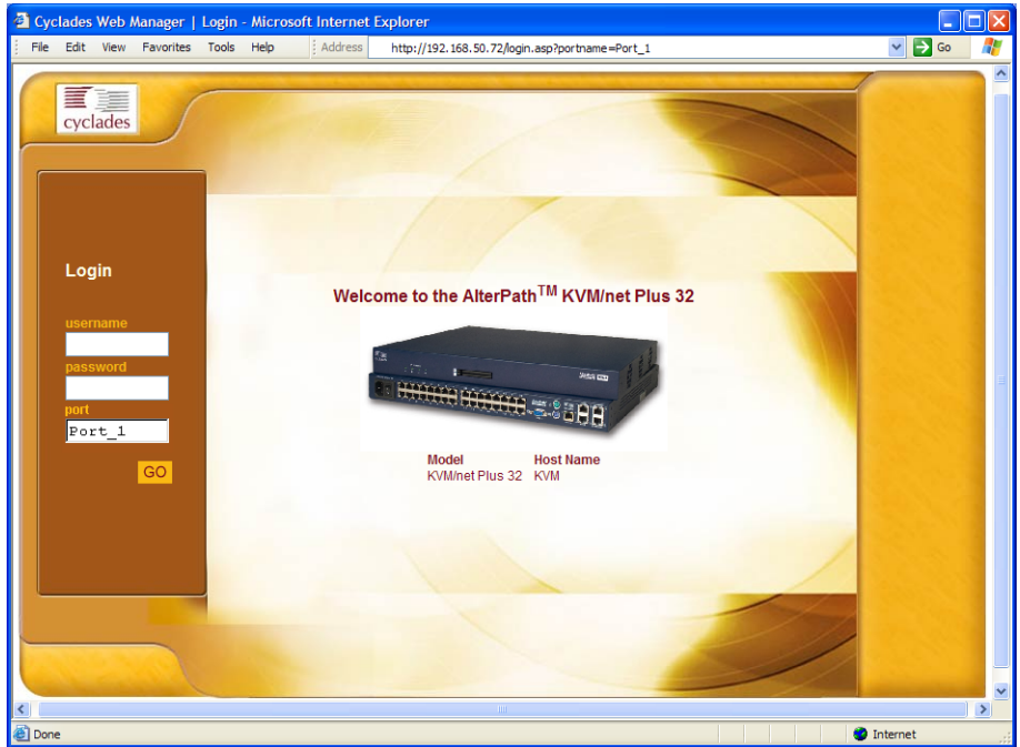
Figure 6-6: Example: Web Manager with Direct Logins Enabled, IP Address and Port Entered
