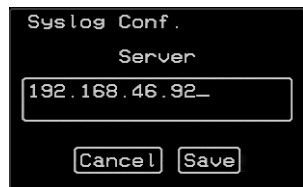
Figure 7-8: Syslog Configuration Server Screen
