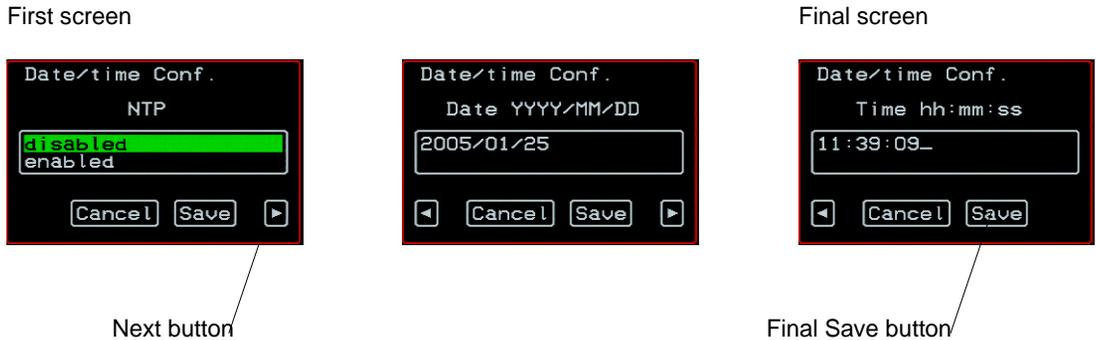
**Figure 7-2:** First, Middle, and Last Screens in Configuration Series
