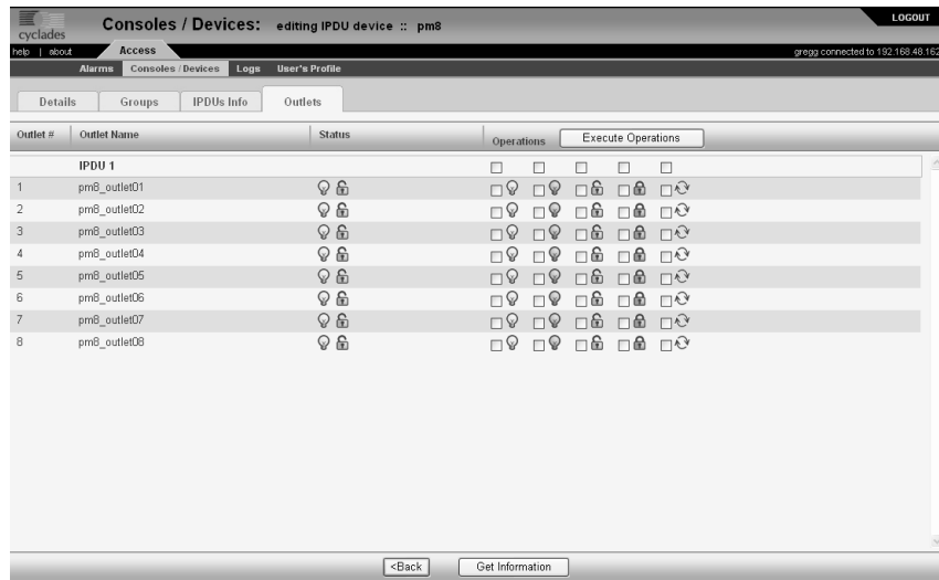
Figure 3-22: PM Device Outlet Control Form
