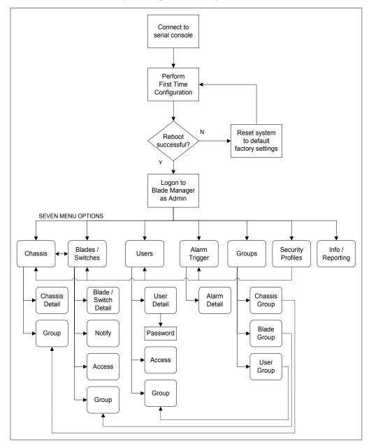
You must perform the First Time Configuration process (see Configuration Flow Diagram) using the command line interface. Once completed, you may perform the rest of the configuration process and all daily administration procedures through the BladeManager web interface.
