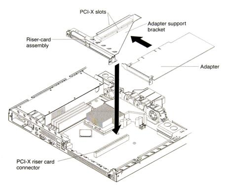
To install an adapter, complete the following procedure:
