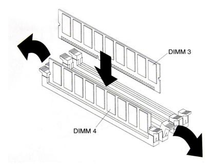
To install a DIMM, complete the following procedure:
