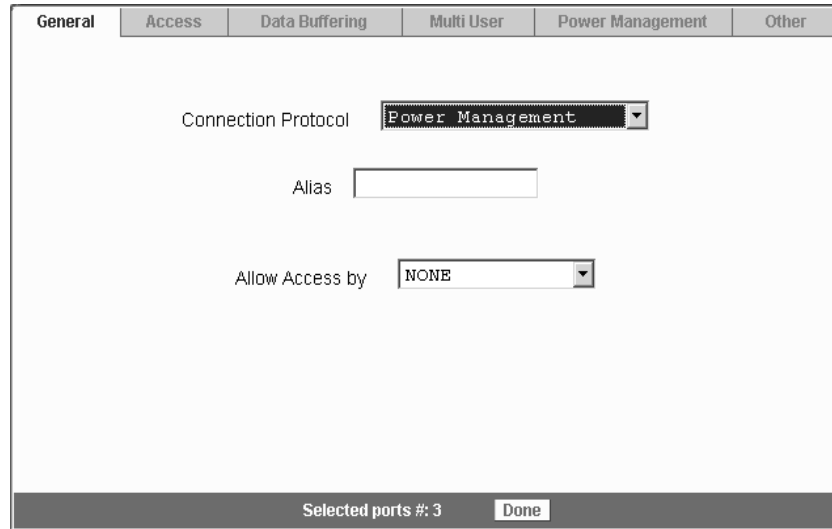
Figure 10-18: Expert > Ports > Physical Ports > Power Management Connection
