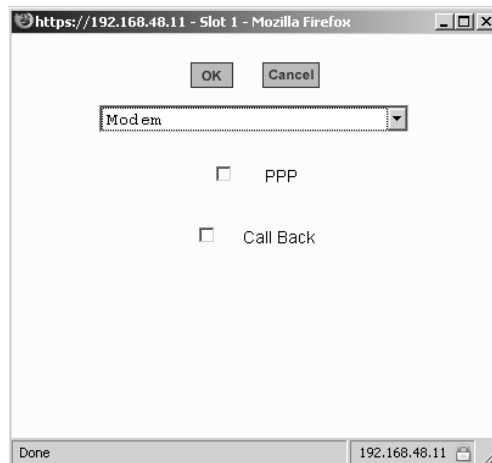
Figure 8-5: Expert > PCMCIA Modem Card Configuration Dialog Box
