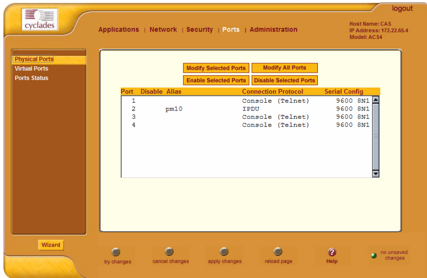
Figure 4-42: Serial Ports Access Modification Form
